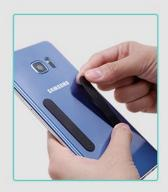
2. Fix the iron sheet on the left and right sides of the phone;
